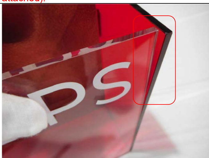
The showcase is cracked (the glue is not firmly attached).
